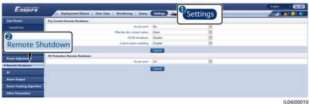
Figure 6-93 Dry contact remote shutdown
