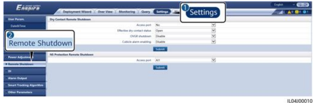
Figure 6-95 NS protection remote shutdown
