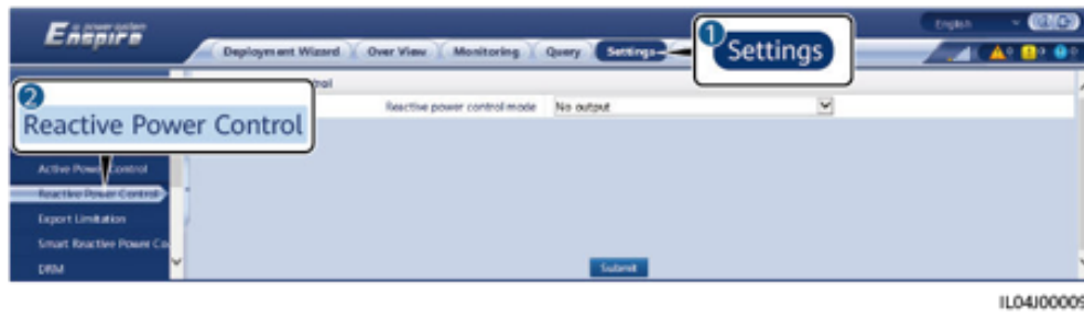
Figure 6-83 Reactive power control
