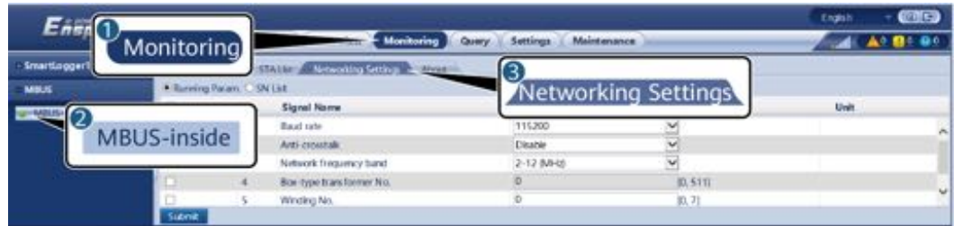
Figure 6-38 Setting the built-in MBUS networking
