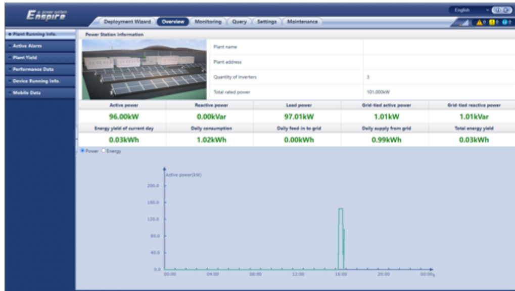
Figure 6-3 Plant running information (with power meter but without battery)
