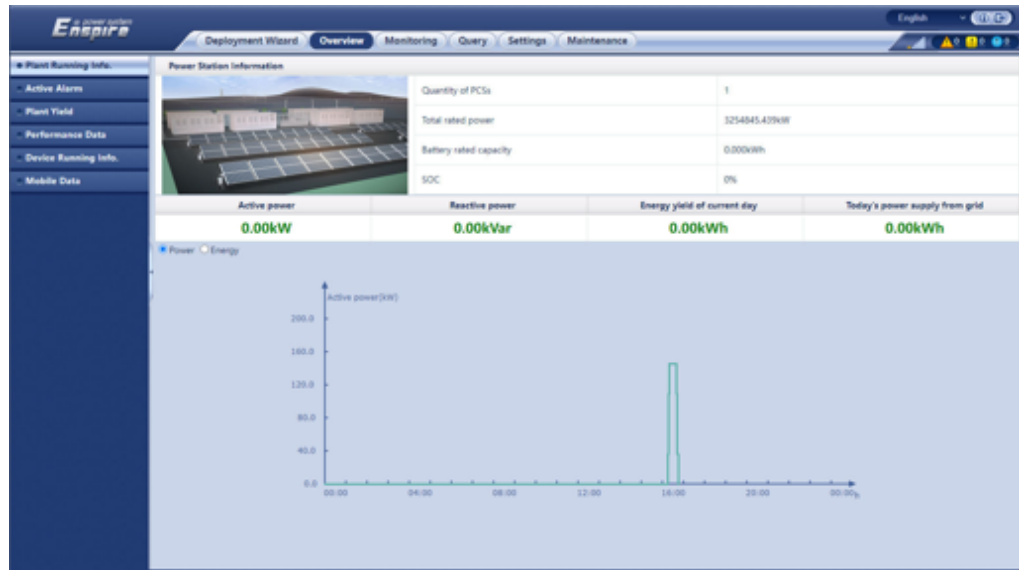
Figure 6-4 Plant running information (with battery but without power meter)
